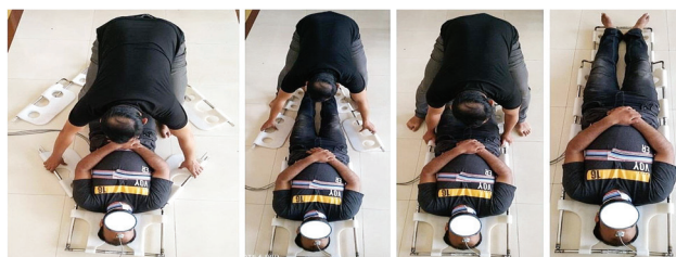
Fig. 2: The developed prototype comprises of multiple segments corresponding to human head, trunk and lower body regions.
