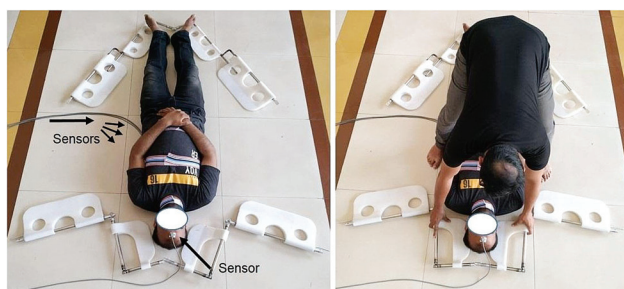
Fig. 3: novel scoop stretcher for full body immobilization during causality transfer.
